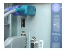
The rectangular socket is a typical USB port. This is often found on the back of a PC, but some manufacturers are also placing them in front for easy access.
