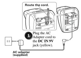
Plug the AC Adapter to a 120V AC power outlet.
