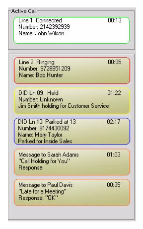
The text box for each call contains the call information includes the calling party information, line being used, and call timer. When the telephone is idle (no active call), the display is empty.
