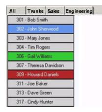
This area of the screen has a button defined for every extension that the user is monitoring. The attendant can define Extension Groups that include a specific set of extensions. The tabs at the top of the BLF Panel represent all of the defined Extension Groups. Selecting a different tab allows the attendant to view only the extensions that are included in that group.
